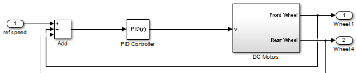
FIGURE 25 SHOWS A BLOCK DIAGRAM OF THE IMPLEMENTATION OF THE PID CONTROLLER AND DC MOTORS
