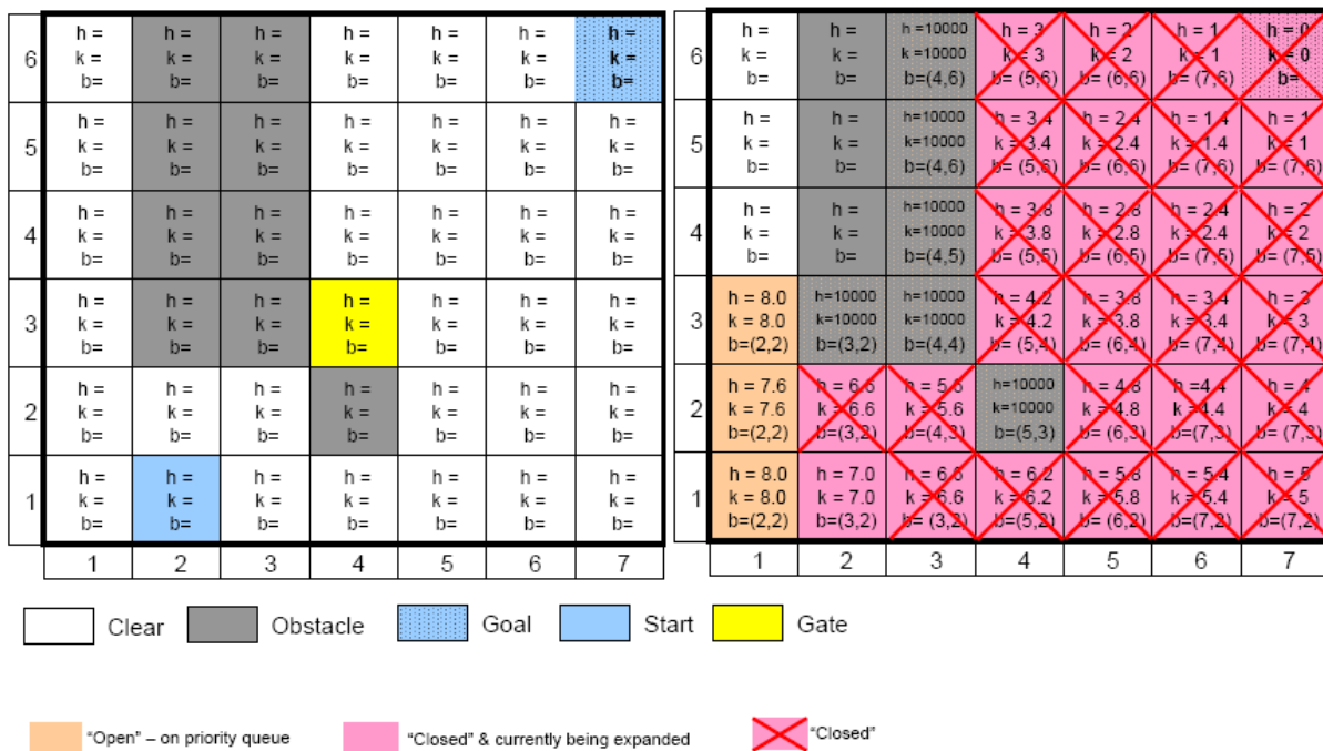
FIGURE 6 DSTAR AREA MAP (LEFT) AND BEGINNING OF THE PATH SEARCH (RIGHT)
