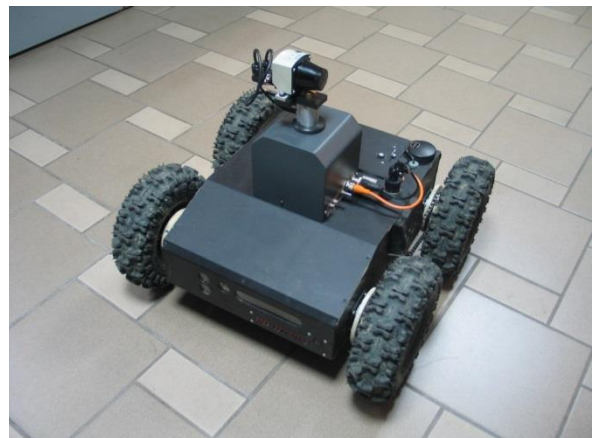
FIGURE 1 THE ROBOTIC PLATFORM DR. JAGUAR 4x4 WHEEL
