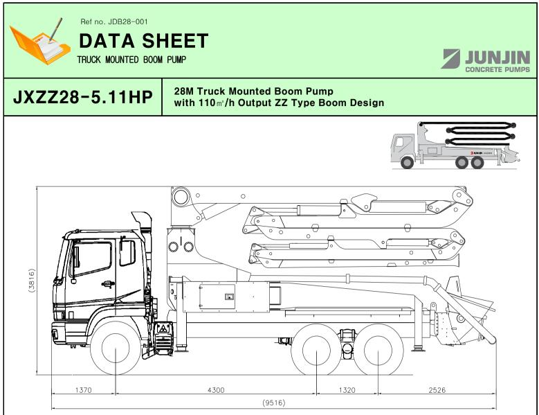
\* Remark : Standard specification with FUSO 6X4. Dimension depends on truck specification.
