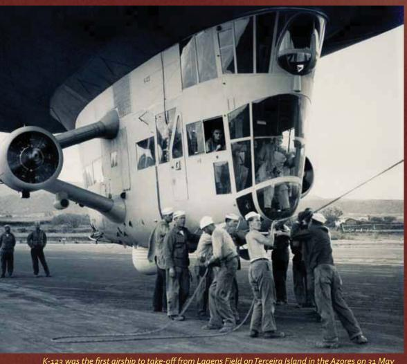
K-123 was the first airship to take-off from Lagens Field on Terceira Island in the Azores on 31 May 1944. Lt. j.g. Homer Bly (pilot) manned the elevator (top right in the control car), Ens. Warren Ireland (co-pilot) manned the rudder (window, top left), and Ens. William Kaiser (co-pilot) took the forward lookout position. (Photo from William Kaiser)
