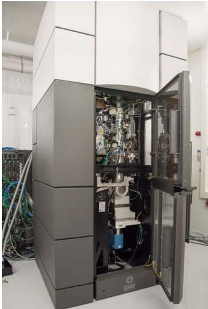
The cryo-EM grid will be loaded first in a Polara electron microscope equipped with a last generation direct electron detector (IBS). Some images and movies will be acquired. Advantages and disadvantages of direct electron detector compared with CCD camera will also be discussed.
