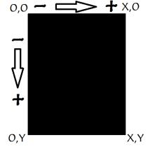
This image shows a PORTRAIT orientation of the screen, the upper left corner is 0,0 (zero,zero). The maximum values of the SMART GPU 2 in PORTRAIT mode are X:271,Y:479.
