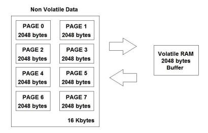
The internal 2048 RAM buffer is used to perform **single byte** read-write operations, once data is ready to be saved, contents of all EEPROM RAM Buffer must be saved on the EEPROM-FLASH Page 0-7. A typical EEPROM-FLASH usage procedure example is described next:
