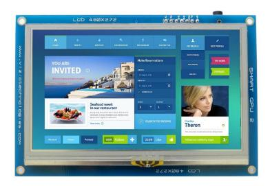
The Smart GPU 2 is a powerful easv use. to intellectual property, embedded graphics. audio and touchscreen processor in a state-of-the-art ARM Cortex-M3 chip; this is mounted on a board with a touchscreen color LCD. lt's aimed to developers to create advanced Graphical User Interfaces (GUIs) in a very easy way. It features high end FAT format data management functions (Data Logger) to create even
