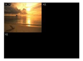
All data is in hex. Note: See that X2 is the sum of X1+(width in pixels - 1), the -1 in the pixels is because pixel number 0 also count. Also Y2 is the sum of Y2+(height in pixels - 1) because the same reason as X2.
