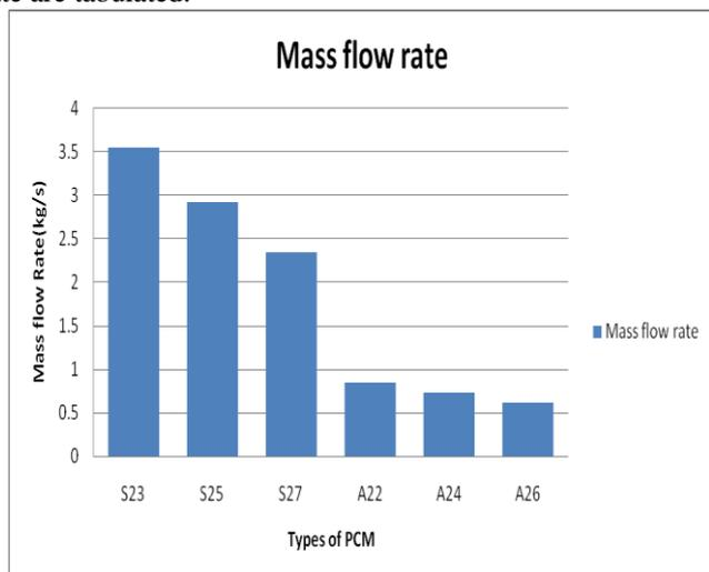
Fig 4 Types of PCM vs. Mass flow rate
