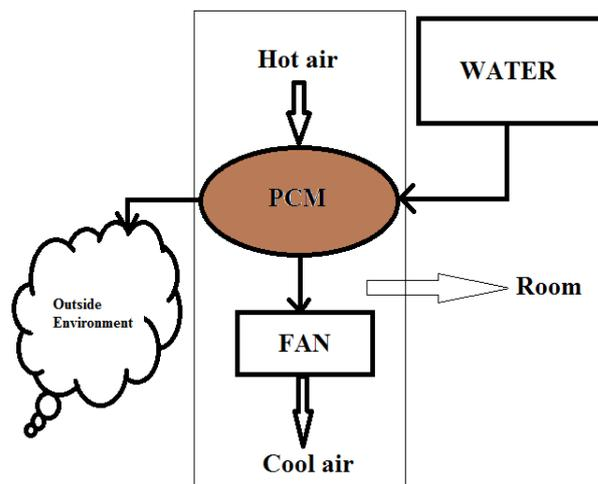
Fig 2 Overview of the cooling system
