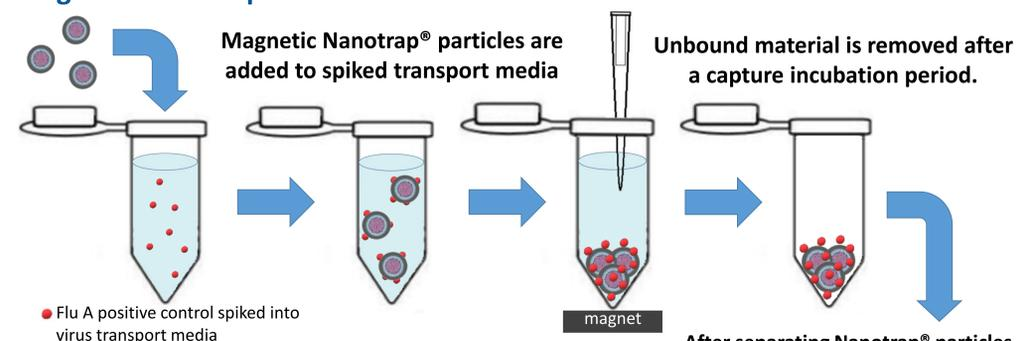
Nanotrap® particle method outperforms QIAGEN columns for extraction of Flu A RNA from spiked samples
