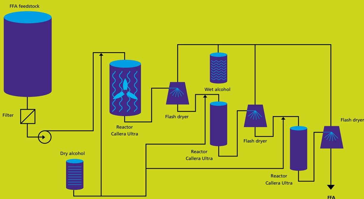
Fig. 10. Continuous biodiesel production from FFA using packed-bed reactors loaded with the immobilized lipase Callera™ Ultra IM produced by Novozymes.
