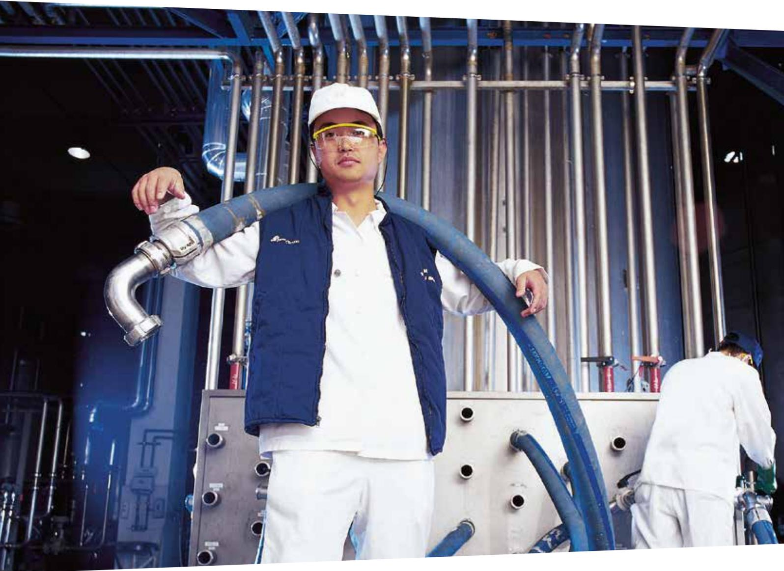
At Novozymes, industrial enzymes are produced using a process called submerged fermentation. This involves growing carefully selected microorganisms (bacteria and fungi) in closed vessels containing a rich broth of nutrients (the fermentation medium) and a high concentration of oxygen (aerobic conditions). As the microorganisms break down the nutrients, they produce the desired enzymes. Most often the enzymes are secreted into the fermentation medium.
