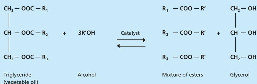
Fig. 9. Transesterification reaction of triglycerides.
