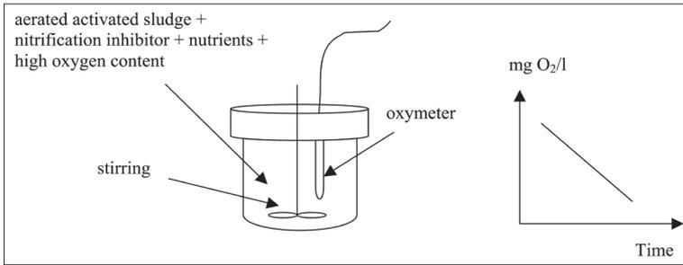
Figure 1. Illustration of the principle of the OUR measurements.
