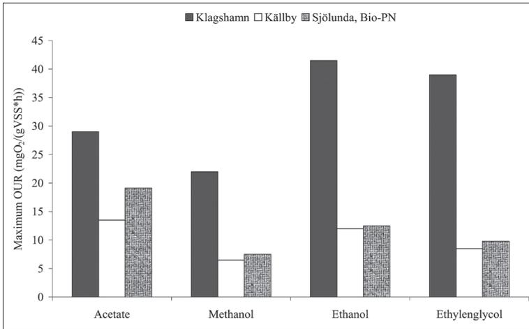
Figure 7. Oxygen uptake rates were measured in sludge from three municipal wastewater treatment plants, while additions of acetate, methanol, ethanol and ethylenglycol respectively were added as carbon source.
