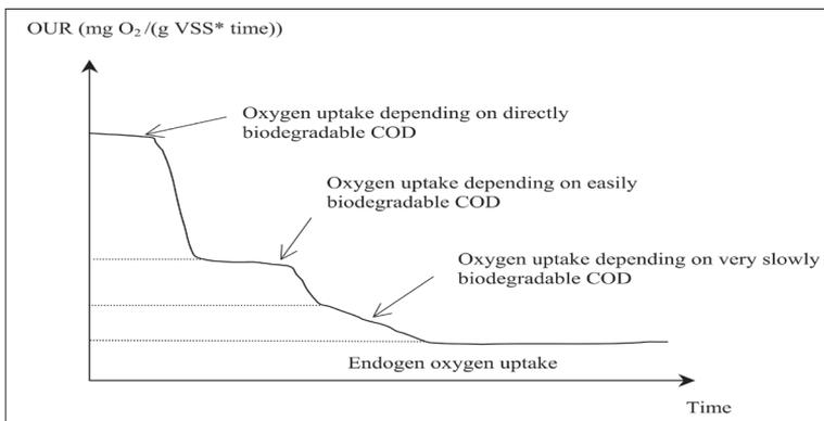
Figure 4. Typical development of the respiration rate as a function of time for a mixture of carbon sources according to Kristensen *et al.*, (1991).
