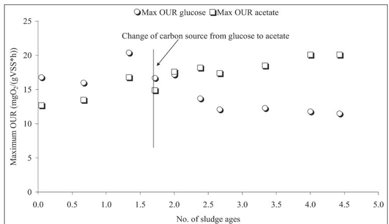
Figure 8. Maximum oxygen uptake rates for acetate and glucose were followed in activated sludge exposed to glucose in the first period and acetate in the second period (Hagman, 2003).
