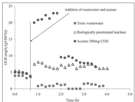
Figure 6. Toxicity test. Three parallel respiration tests, one with additions of acetate, one with biological pre-treated leachate and one with toxic wastewater. Sludge from the same plant with identical conditions was used in all reactors.
