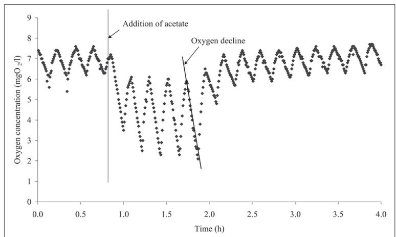
Figure 2. A plot of the oxygen concentration during intermittent aeration of activated sludge from Källby WWTP in Lund. Acetate added after 0.8h.
