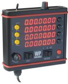
Switch the unit on at the left 2-step switch. The unit is now switched on, recognisable by the red lit digits of the 4 displays.
