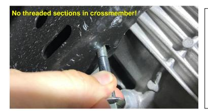
Note: When starting step 8, if there are no threaded sections in the crossmember, you will need to place the provided M8 flange nuts in the crossmember. Place the nuts in the slots that are above and to the left of the crossmember hole. Then using a finger, move into position and hold down the nut when threading the M8 bolts.
