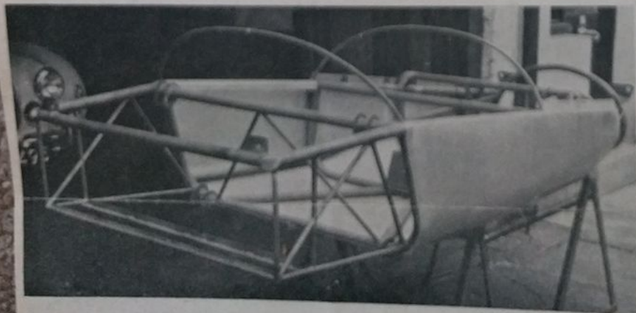
A close view of the Yimkin frame shows the body hoops, stressed sides and undertray.
