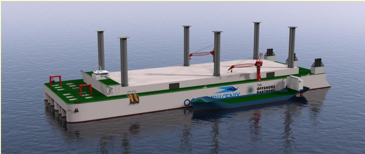
Of trimaran design, it can be subsequently outfitted with 'SWATH' hulls. In a patent protected variant the vessel may be of the single-hulled type.
