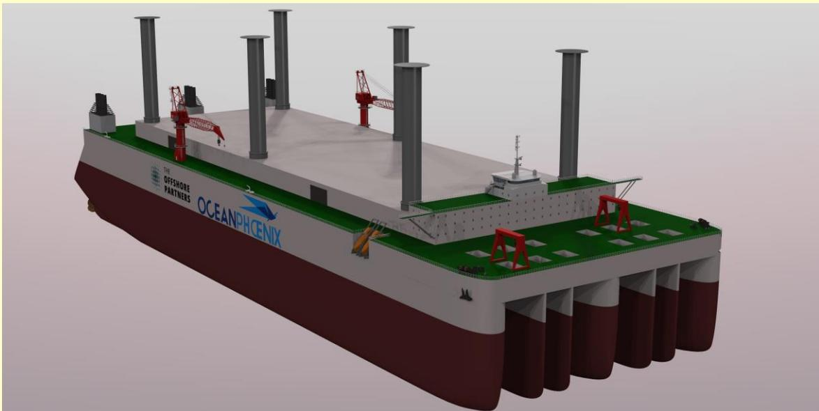
The Ocean Phoenix will retrieve, compress, and pack waste in accordance with road transportation regulations, this taking place before the transferral of the waste to an accompanying support ship that brings it onshore for recycling.
