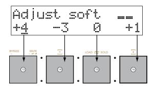
Assuming that the global threshold value for *LEVEL 2* of the 'soft' set is 46, the resulting individual soft thresholds (for *LEVEL 2*) of each one of the four pads will be:
