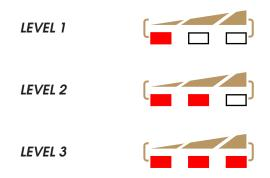
When you apply enough pressure to reach the first threshold level, one LED will light up, indicating that *LEVEL 1* has been activated. Apply enough pressure to reach the second threshold level and two LEDs will light up, indicating that *LEVEL 2* has been activated. When enough pressure has been applied to reach the third threshold level, the full line of three LEDs will light up, indicating that *LEVEL 3* has been activated.
