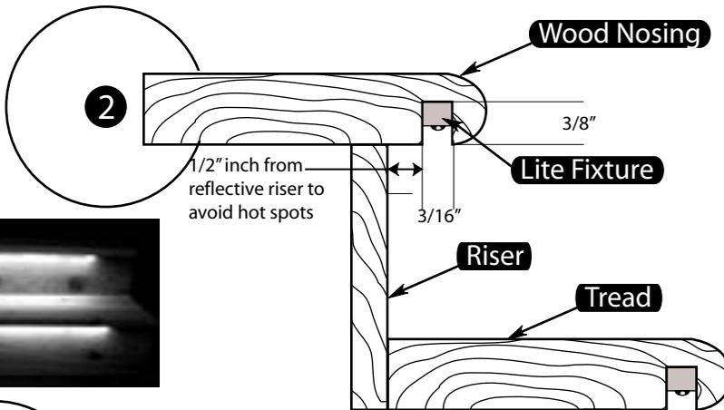
**FOR STAIR INSTALLATION:** [ILLUS. 2] using a table saw or router, cut a 3/16" wide x 3/8" deep channel the full length of the stair nosing. For best results, The LED Strip should be at least 1/2" from stair riser to avoid hot spots.
