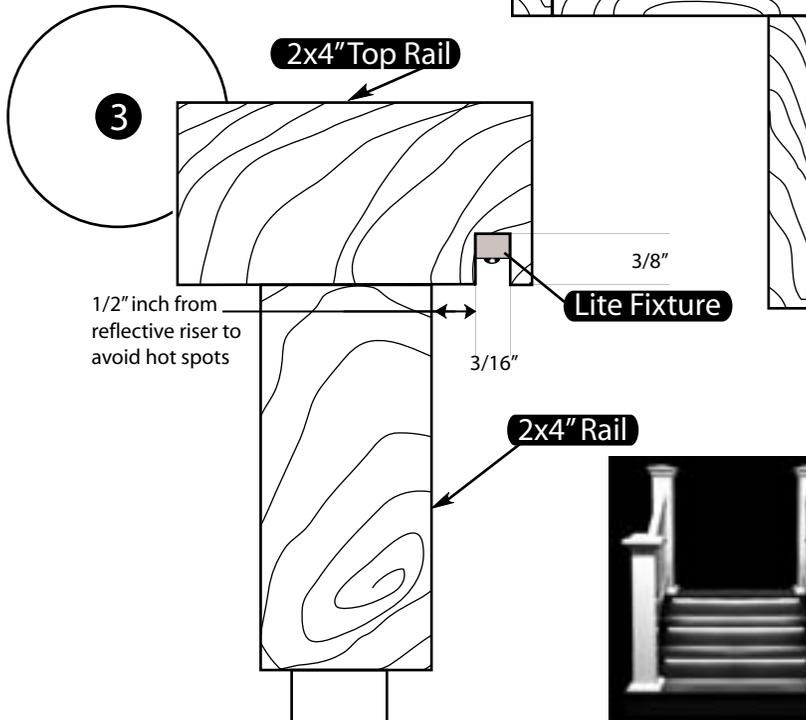
**FOR HANDRAIL INSTALLATION:** [ILLUS. 3] using a table saw or router, cut a 3/16" wide x 3/8" deep channel the full length of the handrail. For best results, The LED Strip should be at least 1/2" from horizontal surfaces to avoid hot spots. The bottom of your hole needs to be flat so the light lays in correctly.
