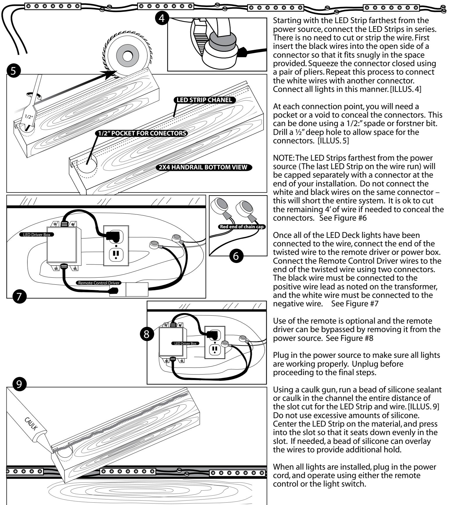
Starting with the LED Strip farthest from the power source, connect the LED Strips in series. There is no need to cut or strip the wire. First insert the black wires into the open side of a connector so that it fits snugly in the space provided. Squeeze the connector closed using a pair of pliers. Repeat this process to connect the white wires with another connector. Connect all lights in this manner. [ILLUS. 4]
