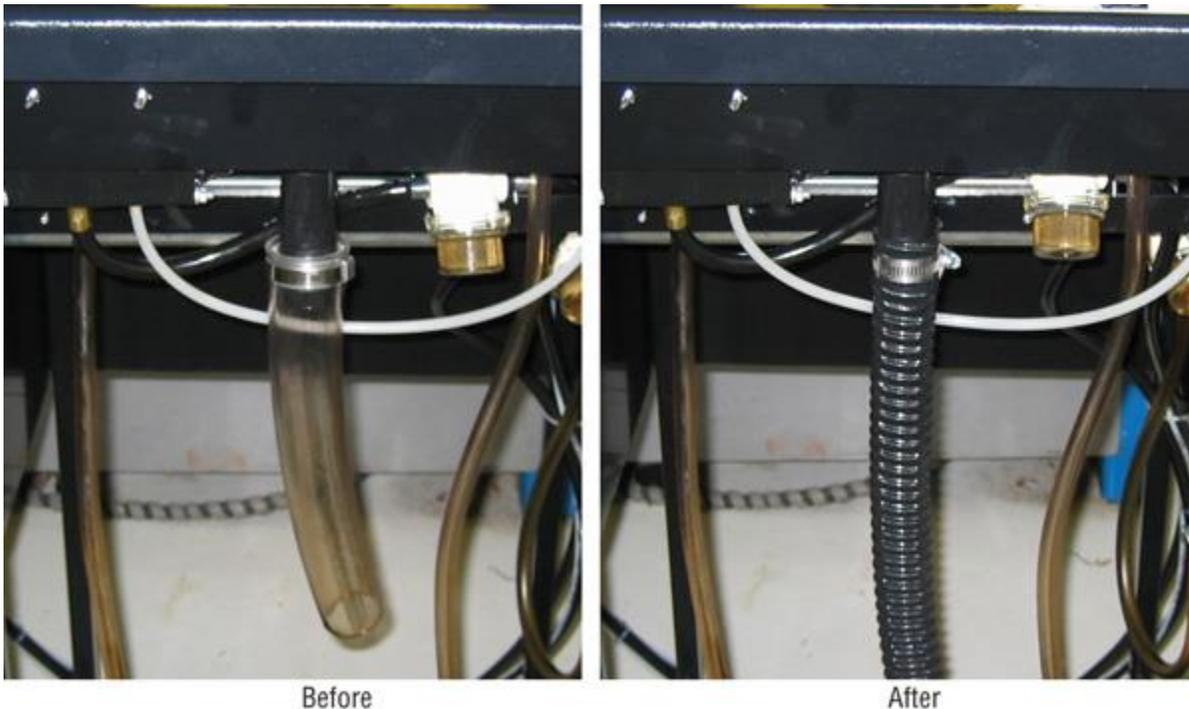
To remove the clear portion of the drain hose simply slide the hose up and pull down. If the hose doesn't pop off after several attempts the clamp must be removed.
