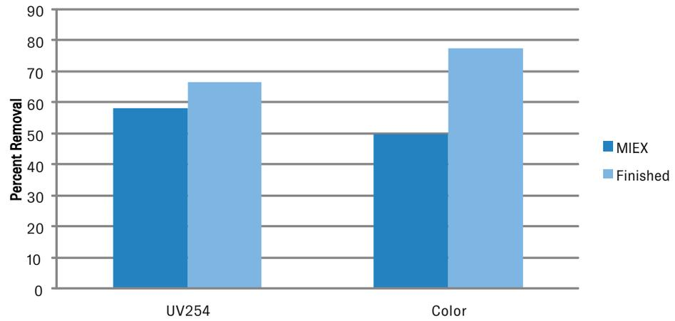
Figure 2: MIEX® TREATED AND FINISHED WATER UV254 AND COLOR REDUCTION
