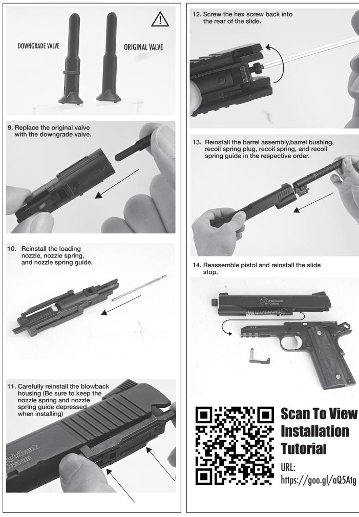
Notice the middle portion of the original valve has no extra material, whereas the downgrade valve has extra material.
