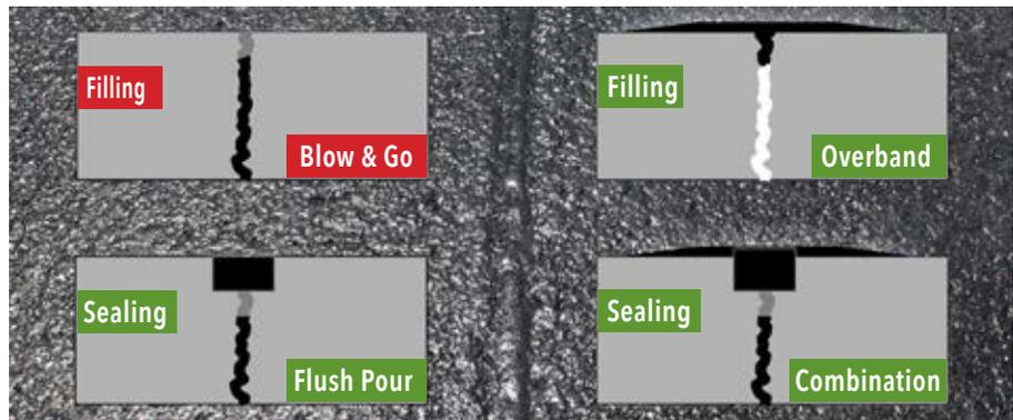
Crack sealing can be performed as a stand-alone process or completed prior to application of quality surface preservation treatments. When properly installed, hot applied crack sealants will last for years to come, protecting your pavement investment. Crack sealing is just one of several integral components in an overall preservation strategy.
