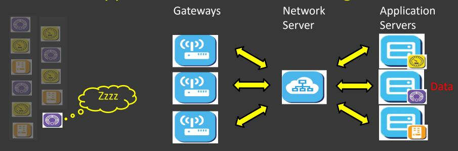
2. However, it has to wait until the Smoke Detector wakes up and transmits a Data Message
