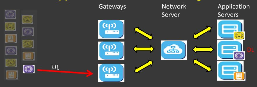
3. When the Smoke Detect transmits, the Data Message moves Upstream
