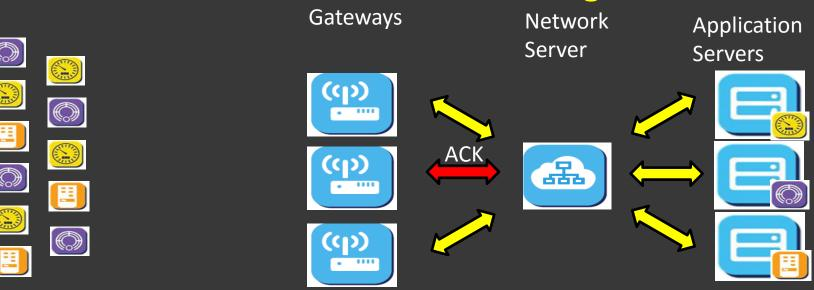
5. The Network Server selects the best path (gateway) to transmit the acknowledgement to the end-device.
