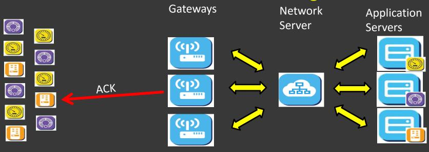
6. The Gateway transmits the acknowledgement to the end-device
