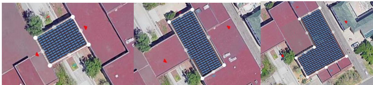
Figure 4: Central Roof PV Mockup using Unirac U-Builder
