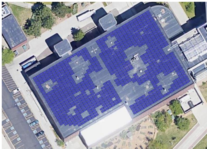
Figure 2: Science Roof PV Mockup using Unirac U-Builder
