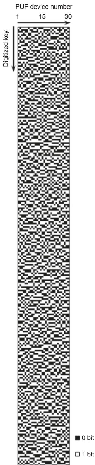
**Fig. 5 Representative binary bitmap of cryptographic keys.** Digitized security keys (256 bits in each PUF) are generated from 30 different edible PUF devices. Notably, the bitstream from this binary bitmap is random, validated by the NIST randomness tests (Table 1 and Supplementary Table 2). The production and fabrication of edible PUF devices are easily scalable due to the choice of materials and the fabrication strategy.
