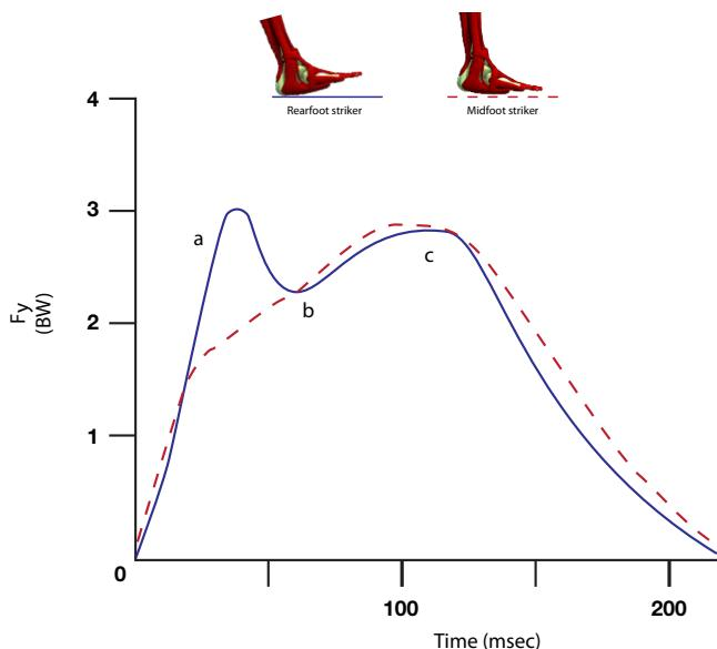
The above graph shows the vertical component of the GRFs for a rearfoot striker and a midfoot striker. There is a larger impact peak (point a) for the rearfoot striker, followed by a slight decrease (b) then a propulsive peak (c).
