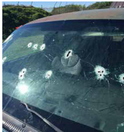
Ballistic testing of the authors preferred ammo configuration on a windshield. (A staggered magazine of FMJ and HP 9mm ammo). The first round always went a little high. FMJ had less of a deviation than HP and ideally you would use the initial hole for followup shots.
