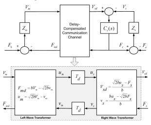
Figure 2. Passivity-based, delay-compensated PEB teleoperation system.
