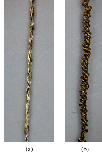
Fig. 1. (a). A conductive nylon thread (V Technical Textiles, 117/17 dtex). (b). A super-coiled polymer (SCP) muscle constructed from coiling the nylon thread in Fig. 1(a).
