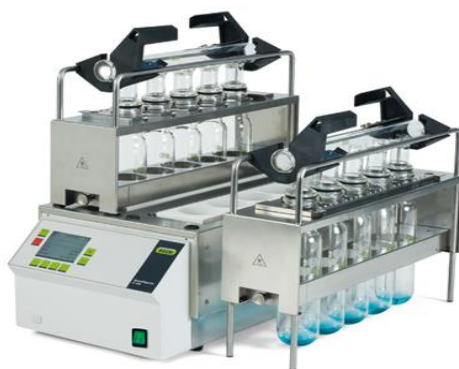
Fig 2. The Kjeldahl apparatus Buchi digester K 436/ K 439 , in which the nitrogen is determined by the amino acid stain (Operation manual SpeedDigester K-425 / K-436)
