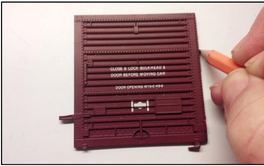
Figure 7. (Left) Using the original door to trace out the Superior door on the back of the styrene "for sale" sign.
