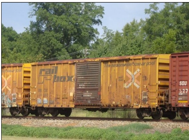
Figure 2 (left). The Youngstown door was the most common style for the prototype... Figure 3 (right). ... as well as for O-scale models of these cars.
