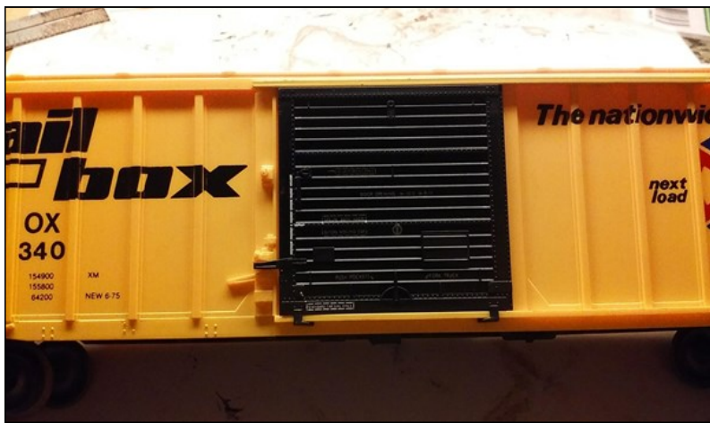
Figure 2 (left). The Youngstown door was the most common style for the prototype... Figure 3 (right). ... as well as for O-scale models of these cars.
