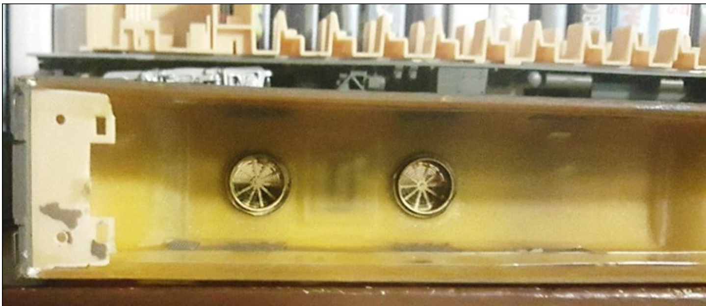
Figure 8. Brass fans are installed. Also, note the mounting tabs with screw holes in them.
