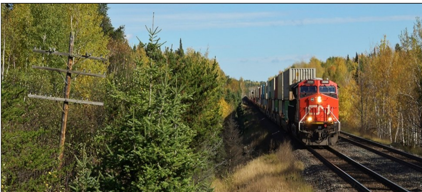
A CN ET44AC leads train X101 through the woods near Wade, Ontario. Note the locomotive's large flared radiators behind the cab.
