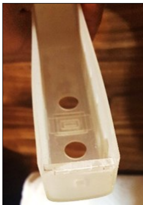
Figure 7 (right). ... and then scribe horizontally across the tabs and flex them until they come loose.
