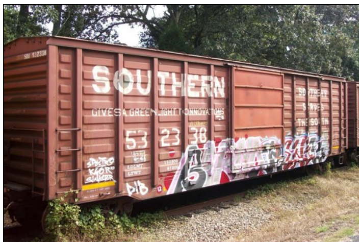
Figure 4 (left). This Southern boxcar has been upgraded to a Superior door. Figure 5 (right). A closer and less angled view of the Superior door.
