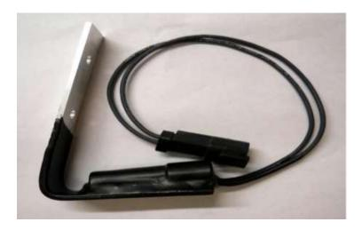
The TILT SWITCH should mount on the side of hood next to the head light assembly.
