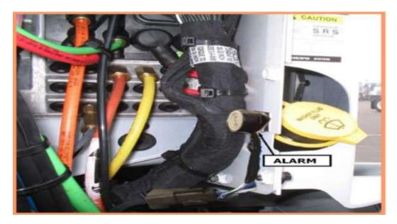
Anywhere in the engine compartment firewall is an acceptable location for installation.
