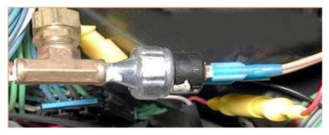
A second switch can be installed on the trailer brakes if desired.
