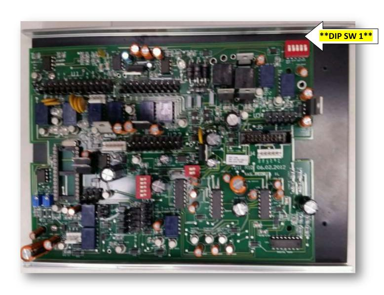
**\*\*DIP SW 1\*\*** CONTROLS THE RPM INPUT FREQUENCY
