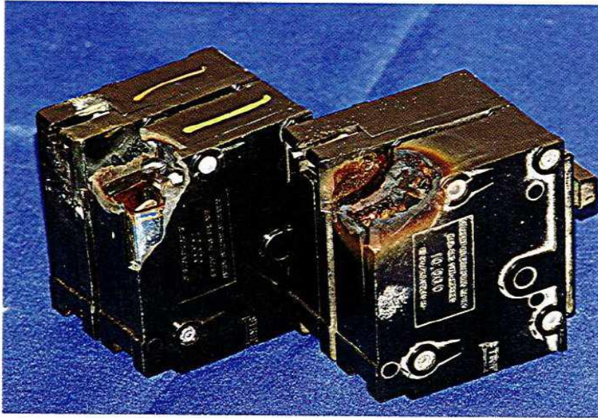
FIGURE 9.10.4(b) Overheated Connections on Two-Pole Circuit Breakers.
