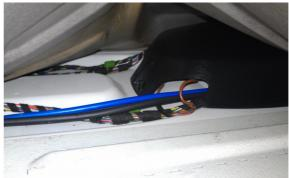
**Long cable set only**: Route the lilac cable under the rubber mat towards the B pillar, following the existing wiring to the seat belt. Drill a14mm hole next to seat belt wiring and fit the supplied grommet. Run the cables through this grommet into the cavity behind the seat belt mechanism and into the voids behind the side panels. Run the cables to where your battery is and proceed as above.
