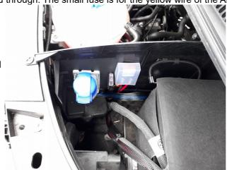
Retrieve enough cable to allow it to pass to the left of the battery and reach to the + terminal of the battery. Using the short bolt from the small plastic bag attach red cable to the battery + terminal.
