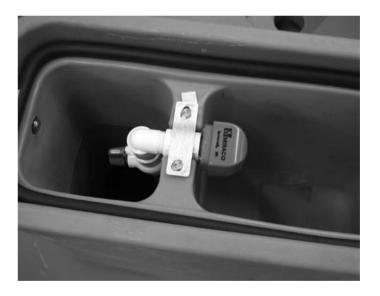
**Step 4**Place the stainless steel bracket over the PVC fitting and attach with 1/4" stainless steel bolts provided.
