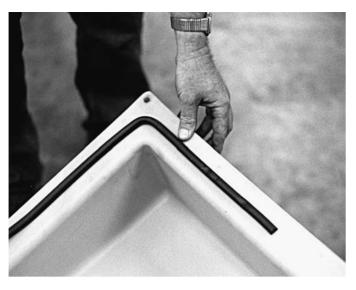
**Step 1**Pull the paper off the back of the rubber gasket and stick to the bottom edge of the tank. This is important to keep out air and water.
