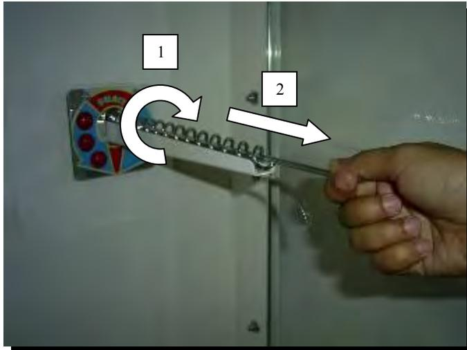
1. Unscrew the Prize Locking pin (**left-hand thread**), by turning it in a clockwise direction.
