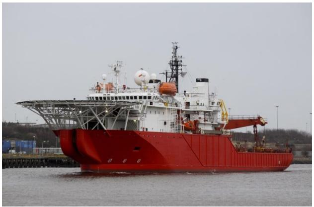
This versatile Saturation Dive Vessel is capable of being employed for various operations worldwide. The advantageous DP2 system in combination with her strong engines making her highly maneuverable at all times. On top she is fitted with multiple thrusters for station keeping and a high level of mobile control
