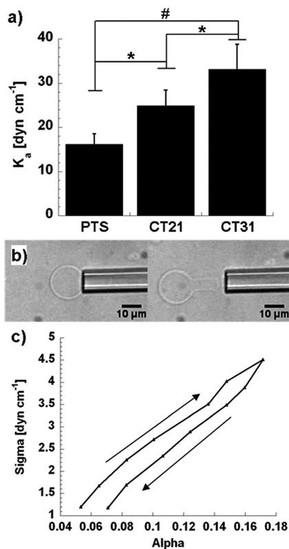
**Fig. 4** Polymersome membrane characterization. (a) Apparent area expansion elastic moduli of giant vesicle membranes measured by micropipette aspiration. PCL membranes are too rigid to be aspirated. (b) A CT31 vesicle immediately before and after release from a micropipette. (c) Typical stress–strain curve for CT31 during micropipette aspiration and injection. The area expansion elastic modulus is calculated from the slope of the curve (up only). \* $p < 0.0005$ , # $p < 0.0001$ .
