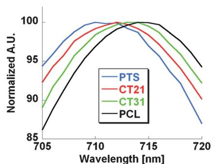
Fig. 5 Fluorescence emission spectra for **PZn<sub>2</sub>** loaded at 2 mol% relative to polymer into nano vesicle membranes.
