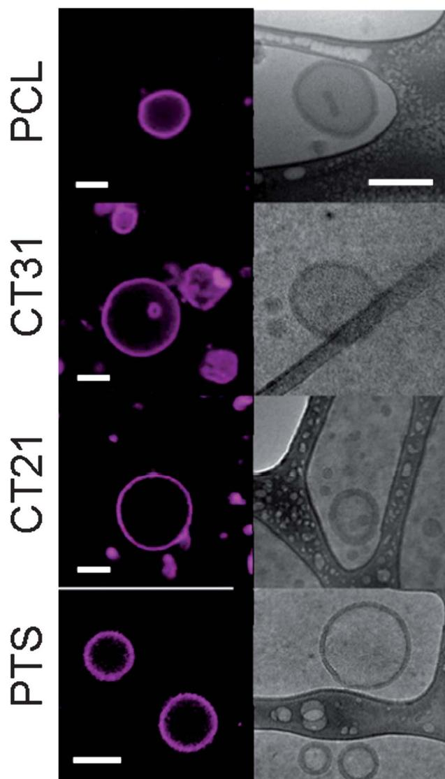
**Fig. 2** Images of polymersomes. Polymersomes of PCL, CT31, CT21, and PTS were imaged by (left) confocal microscopy (giant vesicles) and (right) cryoTEM (nano vesicles). The confocal images show  $\text{PZn}_2$  fluorescence, localized to the membranes of vesicles. Scale bars are  $10\ \mu\text{m}$  for confocal images and  $200\ \text{nm}$  for cryoTEM images.
