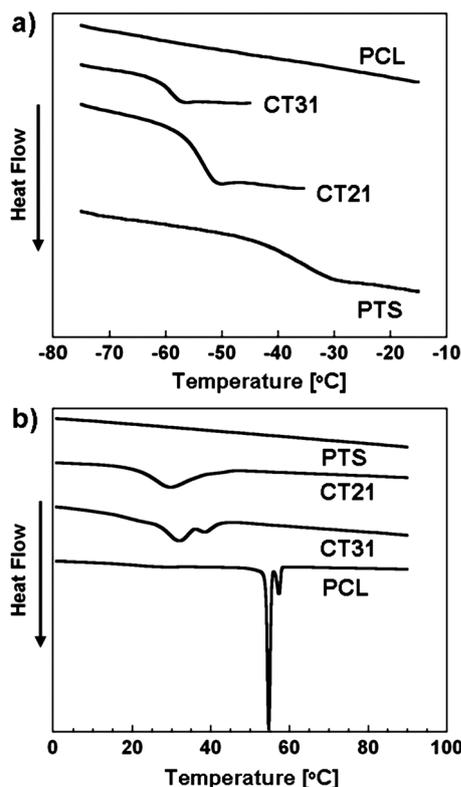
**Fig. 1** Differential scanning calorimetry of diblock copolymers. Heat flow curves showing the (a) glass and (b) crystalline melting transitions for the polymers. The scale of the curve in (a) does not allow visualization of the PCL transition at  $-61.3$  °C.
