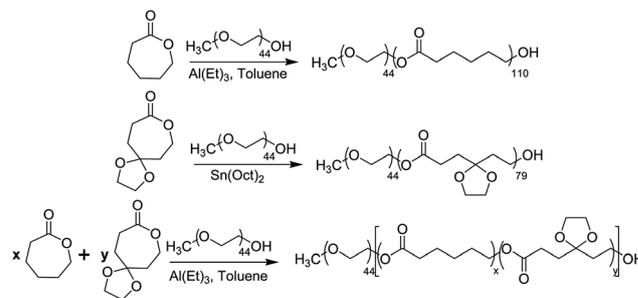
**Scheme 1** Synthesis of PCL (top), PTS (middle), and CT21 and CT31 (bottom). For CT21,  $x, y = 64, 36$ ; for CT31,  $x, y = 77, 23$ .
