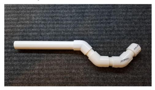
Finally, I inserted the hook arms into the tee fittings. I did not use glue here, so that they could be removed and adjusted or the tee fitting changed if things didn't work out quite right.
