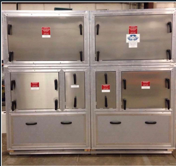
ABOVE: A 60-ton air handler, assembled in the shop for quality assurance testing.
