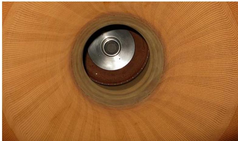
**Figure 5. Internal layer in Silicon Fiber and Phenolic Resin**
