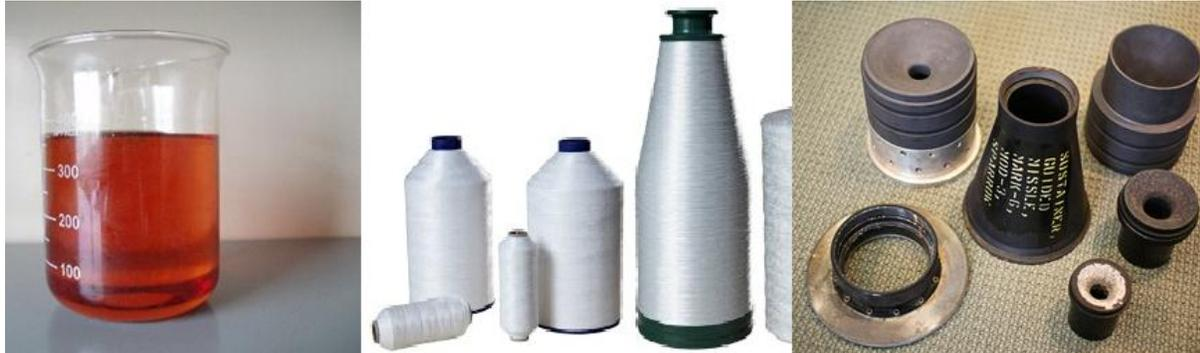
**Figure 6. Phenolic Resin, Silicon Fiber and EDM Graphite**
