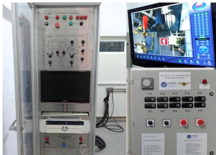
**Figure 12. Control system of the CEU Test Stand**
