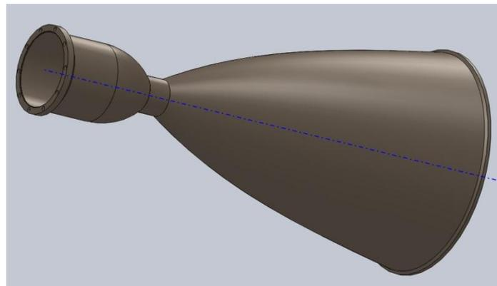
**Figure 8. 3D view of the Metallic Irradiative Chamber**
