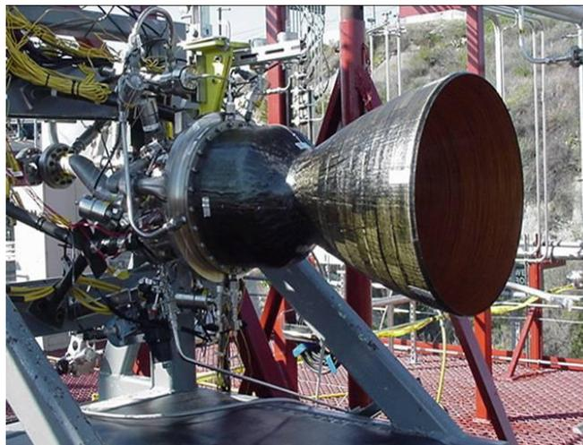
**Figure 3. Ablative engine TR108 of 135kN thrust (KIM, 2005)**
