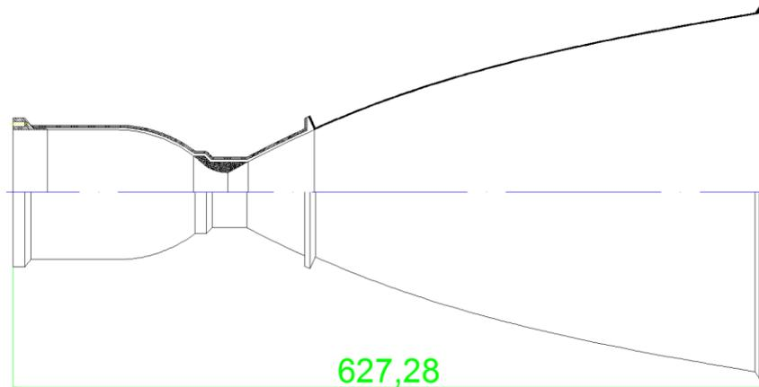
**Figure 9. Ablative Thrust Chamber of 5kN**
