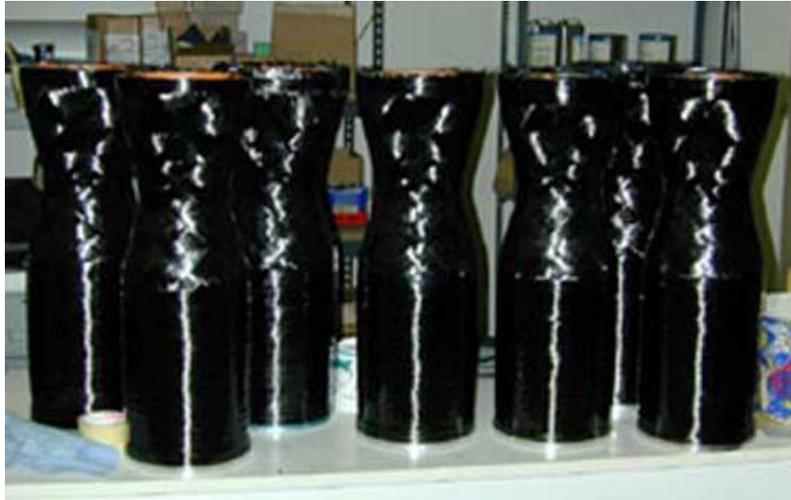
**Figure 2. Ablative engines with 22.5 kN of Thrust from Scorpis Rocket (CONGER, 2002)**
