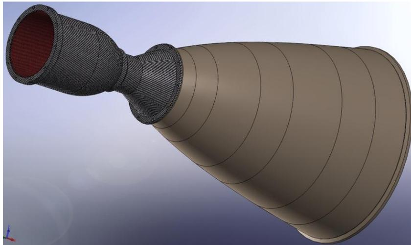
**Figure 10. 3D view of the 5 kN Ablative Chamber**
