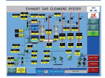
The ECGS is delivered with a PLC based control system (Programmable Logic Controlled) which manages all functionality and provides data logging and storage requirements.
