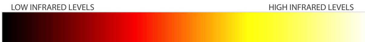
Figure 5: This is the color code for the infrared camera. Infrared has no color, so the color is injected by the computer. The industry standard term for it is "false color".
