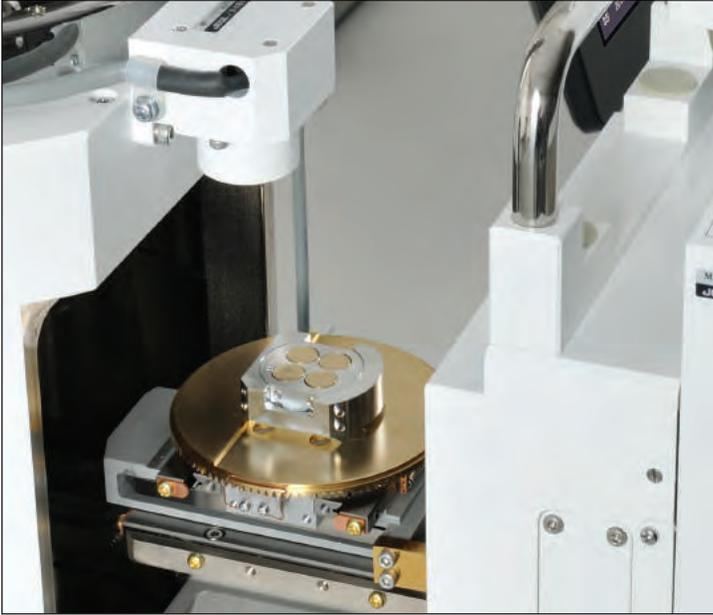
Stage Navigation System camera (optional) and sample stage.
