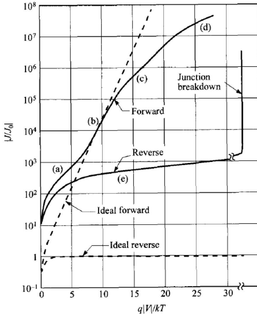
Current-voltage characteristics of a practical Si diode.
