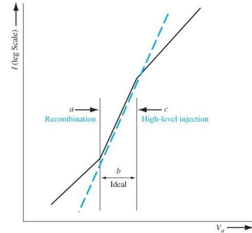
Figure 8.17 | Forward-bias current versus voltage from low forward bias to high forward bias.
