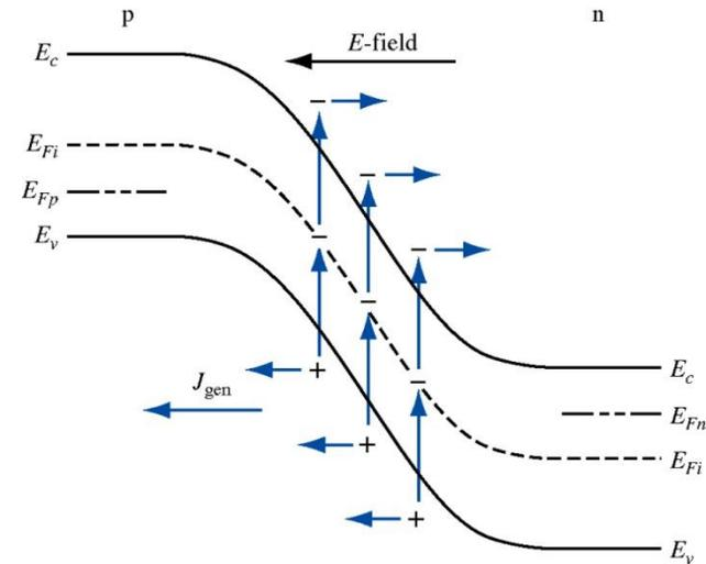
The ideal reverse-saturation current density is independent of the reverse-biased voltage. However,  $J_{gen}$  is a function of the depletion width  $W$ , which in turn is a function of the reverse-biased voltage.
