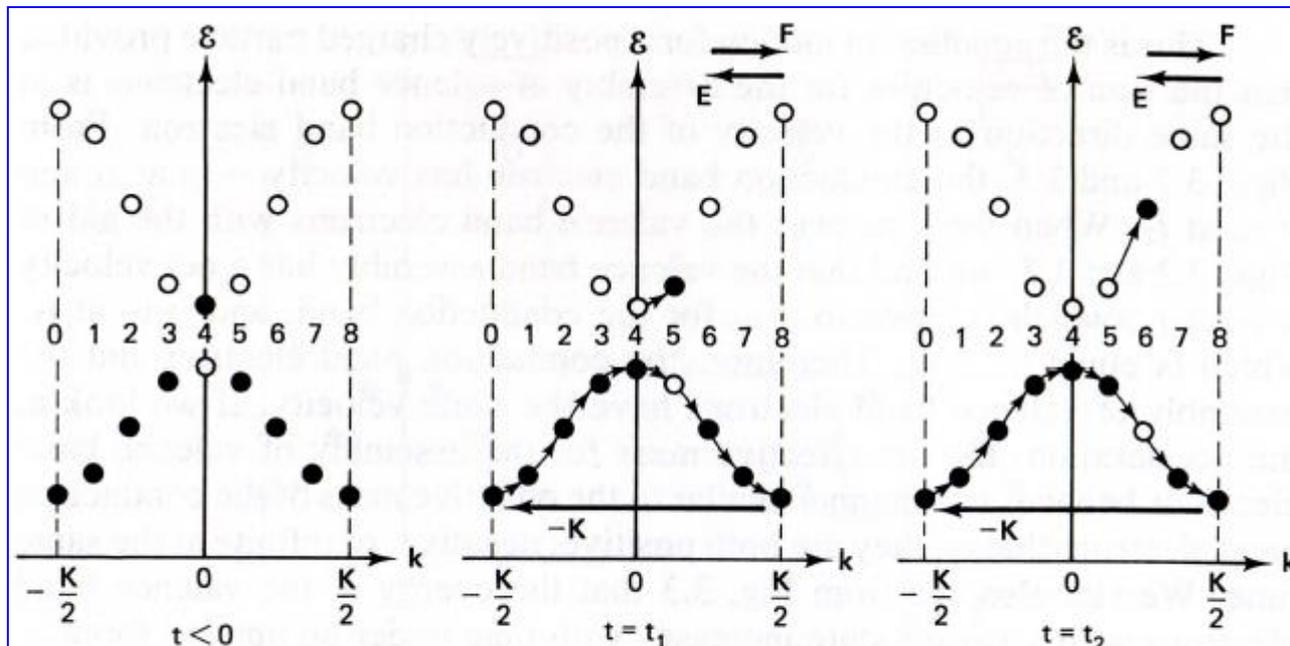
**Figure 3.3** The effect of an applied force on a conduction band with one electron and a valence band with one missing electron.
