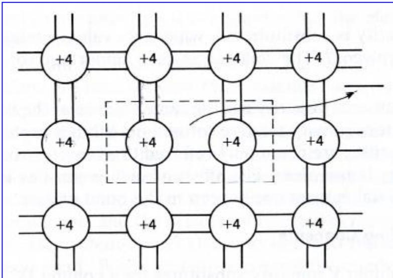
Figure 3.6 (a) Column V substitutional donor impurity and (b) column III substitutional acceptor impurity in Ge.
