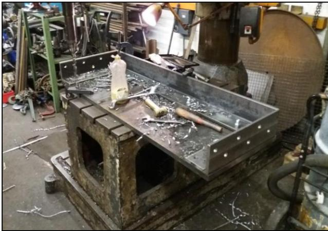
**The picture above shows the mid-frame stretcher on the Radial Drill at Ruddington having the Rivet holes drilled**
