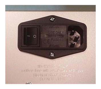
If the EQ doesn't power on after plugging in the power cable and turning the switch to the 'on' position, check to be sure that the fuses are still intact. To do so, unplug the IEC power cable and use a small flathead screwdriver to pop the fuse panel out of the power connector/switch assembly. If either fuse is blown, replace with the same size and type of fuse.
