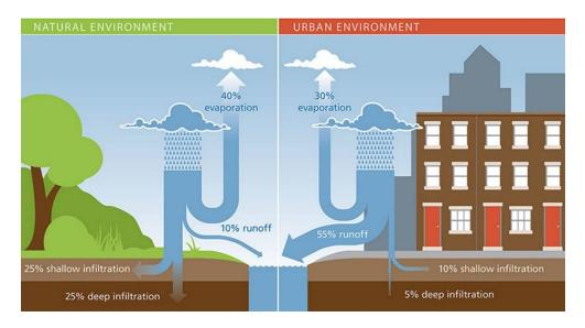
Above is an infographic created by the City of Detroit Water and Sewerage Department, from a Stormwater Management Design Manual published in 2018. It shows the percentage of stormwater as it moves naturally compared to in an urban setting. Presenting information in this way helps us to visualize what those numbers represent.
