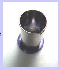
STEP SEVEN: Remove the center bead. Use the 1-inch cutter to cut the second bead smaller. This will allow it to spin inside the ring. Again, centering is very important! If it's not centered, the bead will not spin and will hit on one side of the ring.
