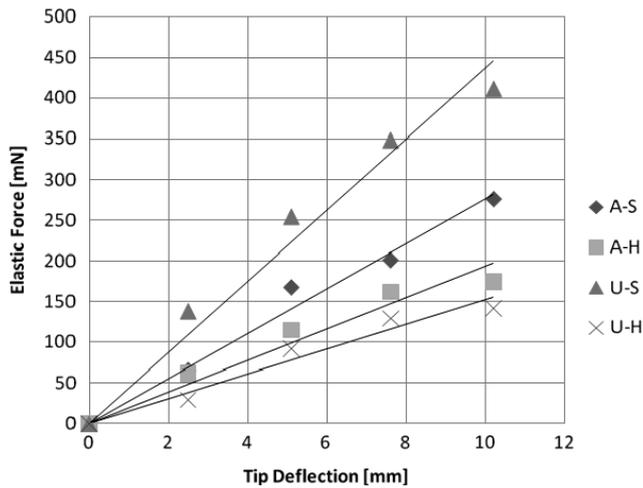
**Figure 7.** Deflection as a function of tip displacement at zero field for all four classes, yielding the elastic compliance,  $\kappa$ .
