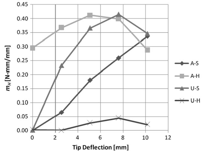
**Figure 8.** Calculated distributed magnetic moment in all four classes for  $\mu_0H = 0.09$  T. Lines are drawn as guides to the eye.
