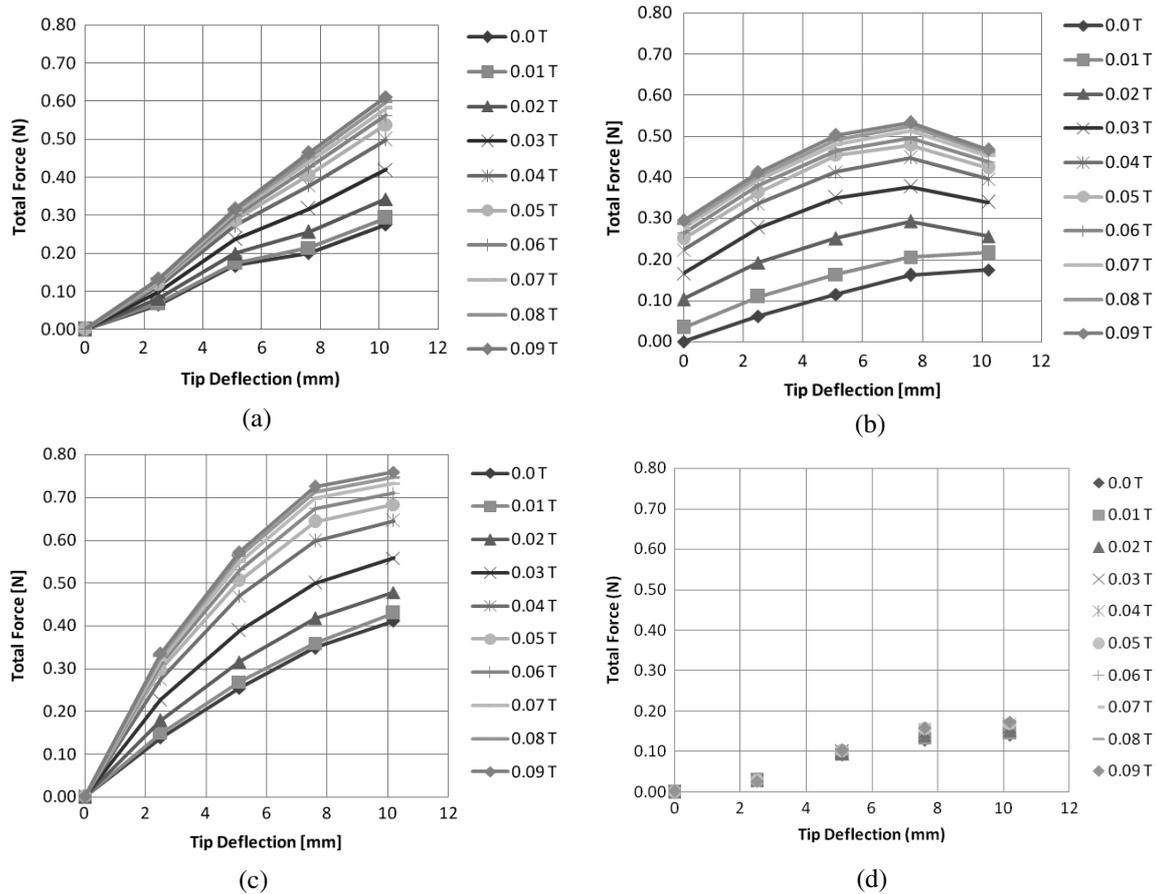
**Figure 4.** Total force as a function of tip deflection for (a) class A–S, (b) class A–H, (c) class U–S, and (d) class U–H. All forces generally increase with field strength and tip deflection; however, for class A–H, there are non-zero forces even at zero deflection.
