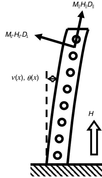
**Figure 10.** Schematic of the cantilever beam showing the nominally aligned particles, parallel and perpendicular component directions of the magnetic field  $\mathbf{H}$ , magnetization  $\mathbf{M}$ , and demagnetizing tensor  $\mathbf{D}$ , transverse bending deflection  $v(x)$  and deflection angle  $\theta(x)$ .
