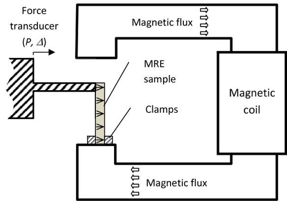
**Figure 3.** Experimental setup of forced displacement testing showing magnetic coil with flux direction. A non-ferrous extension to the force gauge proscribed displacement and recorded the resisting load. The MRE poling direction, if present, is shown by arrows in the sample.
