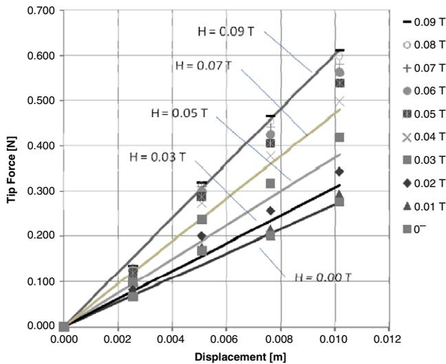
**Figure 11.** Tip force as a function of field and tip displacement for A–S material. The lines represent predictions made with equation (18) based on one adjustable parameter,  $c$ , which depends upon the magnetic susceptibility.
