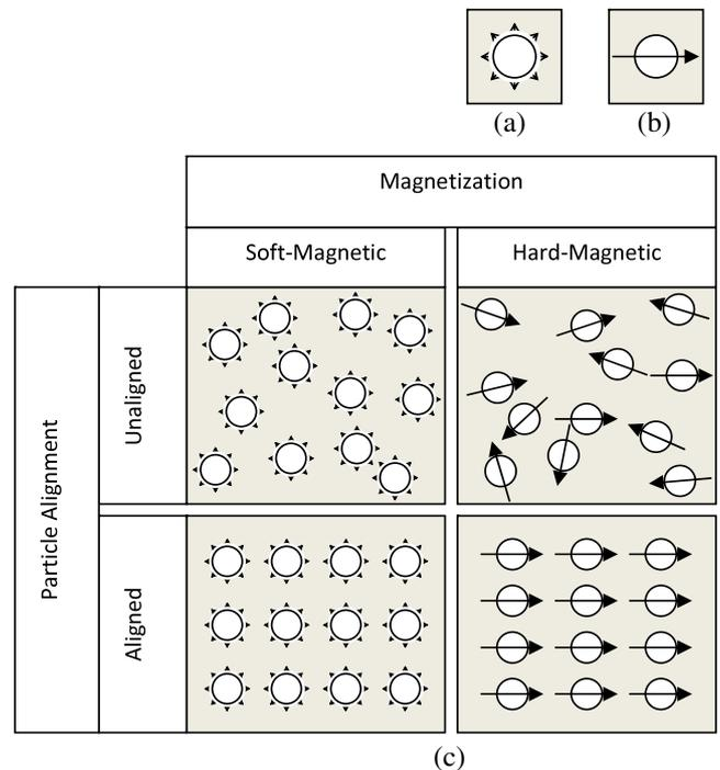
**Figure 2.** Iconography of (a) soft-magnetic and (b) hard-magnetic particles, and (c) schematics of four classes of MREs based on alignment–magnetization permutations.
