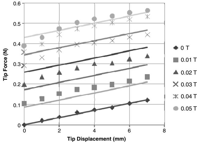
**Figure 9.** Tip force as a function of field and tip displacement for A–H material. The lines represent predictions made with equation (8) based on constants taken from zero field (diamonds) and zero tip displacement ( $y$ -axis) cases.
