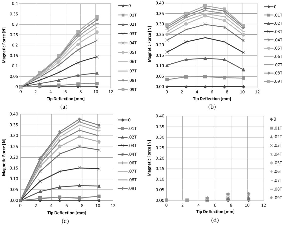
**Figure 5.** Magnetic force as a function of tip deflection data for (a) class A–S, (b) class A–H, (c) class U–S, and (d) class U–H. Forces for classes A–S and U–S are initially linear with respect to displacement and scale with the field. Class A–H is the only class capable of exerting force at zero tip deflection while forces in class U–H are significantly smaller than those of other classes.
