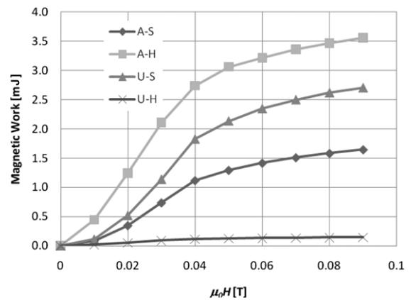
**Figure 6.** Magnetic work done as a function of field for all four classes.
