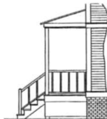
Above: Inappropriate. Balusters are too far apart.
