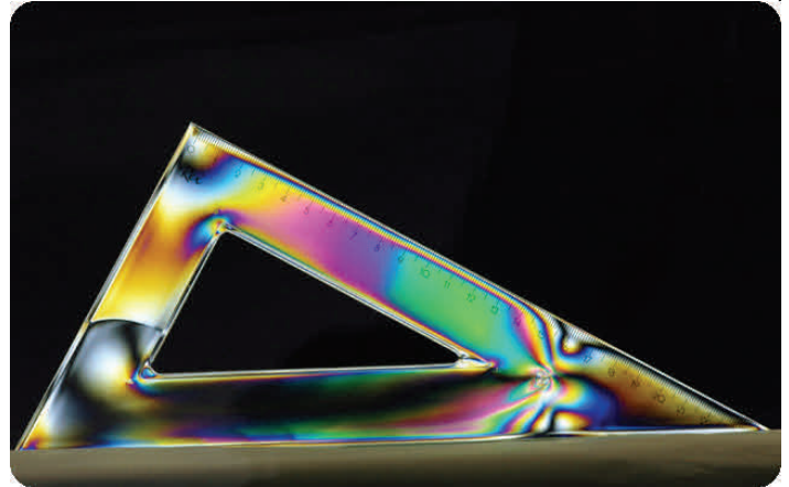
Residual Stress Patterns in Common Objects
